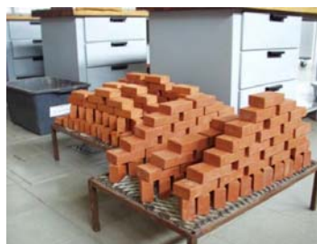
Figure 5 Bricks after the firing process
