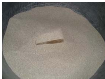
Figure 4 Sand-coating of newly made bricks
