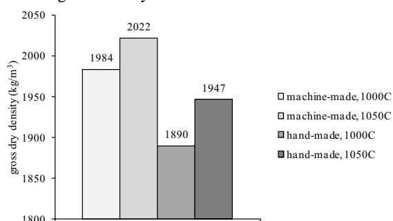
Figure 10 Results of gross dry density testing
