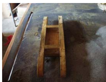
Figure 3 Mould for handmade bricks
